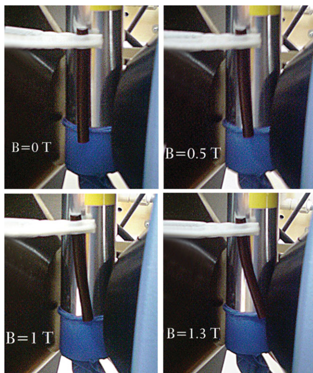
Figure 7 The photographs taken during the bending process under magnetic field of the ferrogel. The values of magnetic field are given in the photographs. [Color figure can be viewed in the online issue, which is available at www.interscience.wiley.com .]
